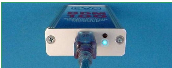
Pict 2: The BSL-module is always connected to the USB cable first.
