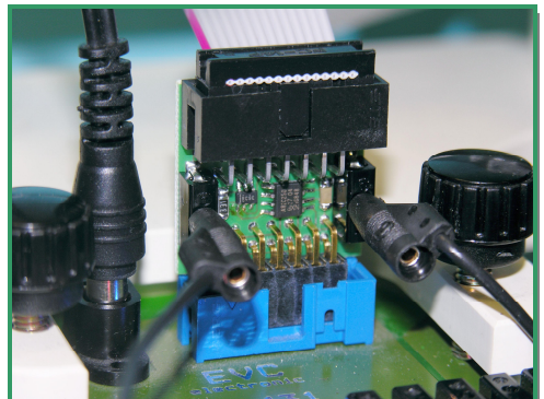
Pict 2: Detailed view of the BSL-DRV module. In this case it's plugged to a BSL131 probe.
