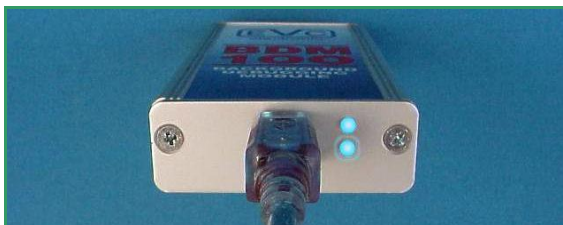
Pict. 3: The BSL100 has established a data connection to an ECU.
