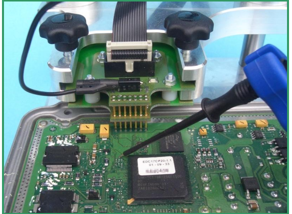
Pict.1: The BSL130 probe is lowered to the pad array and the bootpin probe is placed on the bootpin.
